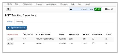
To mark a device as inactive, uncheck the check-box next to Active > Inactive devices are not able to be assigned to patients on the Tracker tab > To add a device to the clinic inventory, tap **Register New Device** > A new row will be added to the top of the table > Type in the Device ID (required), Manufacturer, Model, Serial Number, and EE Number > Tap the floppy disk icon to save and add the device to the clinic inventory. To discard any information you entered, tap **X**.
